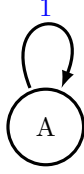
FIG. 18. Biased coin process \epsilon -machine, when \beta converge to negative infinity and p < 0.5 , or when \beta converge to infinity and p > 0.5 a deterministic process
